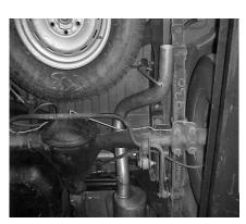
INSTALL OVERAXLE TAILPIPE #C TO THE OUTLET OF THE MUFFLER USING HANGER #G. INSERT WELDED HANGER INTO RUBBER GROMMET.
