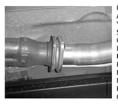
UNBOLT THE STOCK EXHAUST AT THE FLANGE BEHIND THE Y-PIPE AND REMOVE. MAKE SURE TO LEAVE ALL RUBBER GROMMETS IN THE FACTORY LOCATION. YOU WILL RE-USE STOCK NUTS, BOLTS. FOR EASIER REMOVAL OF EXHAUST, CUT BEHIND THE MUFFLER. USE WD-40 TO REMOVE HANGERS FROM GROMMETS.
