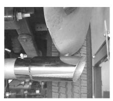
INSTALL THE STAINLESS STEEL TIP NOW; FIRMLY TIGHTEN EVERYTHING ALL CLAMP, HANGERS, BOLTS AND FLANGE. TO CLEAN TIP USE ANY STAINLESS OR ALUMINUM CLEANER WITH A SCOTT BRITE PAD.
