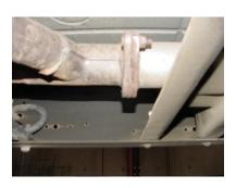
TO REMOVE STOCK EXHAUST UN-BOLT THE FACTORY FLANGE LOCATED IN FRONT OF THE MUFFLER. DO NOT THROW AWAY THE STOCK BOLTS AND NUTS. YOU WILL RE-USE THEM. LEAVE ALL RUBBER GROMMETS IN PLACE. USE WD-40 TO AID IN REMOVAL OF THE STOCK EXHAUST AND HANGERS.
