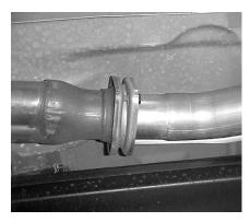
UNBOLT THE STOCK EXHAUST AT THE FLANGE BEHIND THE Y-PIPE AND REMOVE. MAKE SURE TO LEAVE ALL RUBBER GROMMETS IN THE FACTORY LOCATION.
