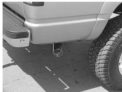
INSTALL STAINLESS STEEL TIP. TO CLEAN YOUR TIP USE ANY STAINLESS OR ALUMINUM CLEANER. TIGHTEN ALL CLAMPS, HANGERS AND CHECK FOR LEAKS.
