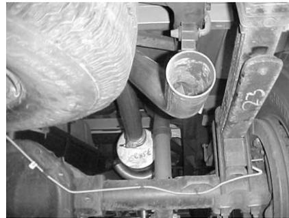
INSTALL OVERAXLE TAILPIPE #D INTO REAR OF MUFFLER NO MORE THAN 1 1/2" TO 2". INSERT WELDED HANGER INTO RUBBER GROMMET. DO NOT TIGHTEN. USE CLAMP #H TO ATTACH TO MUFFLER.
