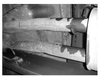
LAY OUT THE GIBSON EXHAUST SO IT LOOKS LIKE THE DRAWING AND COMPARE THE PART NUMBERS. FOR AN EASIER REMOVAL OF THE FACTORY EXHAUST CUT THE TAILPIPE BEHIND THE MUFFLER. THEN CUT 18" IN FRONT OF THE FACTORY MUFFLER AND REMOVE. LEAVE ALL FACTORY RUBBER GROMMETS IN PLACE.
