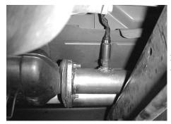
RE-INSTALL O2 SENSOR. USE A SMALL AMOUNT ANTI- SEIZE ON THE THREADS. NOW FIRMLY TIGHTEN ALL CLAMPS, HANGERS, FLANGE, AND BOLTS
