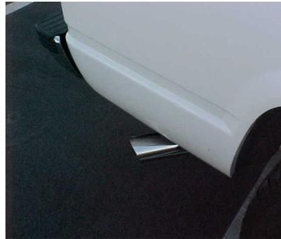
INSTALL TURNOUT PIPE #D INTO TAILPIPE USING CLAMP #G . INSTALL THE STAINLESS TIP AND CLAMP DOWN. USE ANY STAINLESS STEEL OR ALUMINUM CLEANER TO POLISH TIP.
