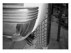
INSTALL TURNOUT PIPE #D INTO TAILPIPE USING CLAMP #G . INSTALL THE STAINLESS TIP AND CLAMP DOWN. USE ANY STAINLESS STEEL OR ALUMINUM CLEANER TO POLISH TIP.
