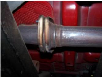
2. To remove the stock exhaust, unbolt it at the 2-bolt flange in front of the muffler. Disengage the welded hangers using WD-40 from the OEM rubber grommets. Do not damage or remove the rubber grommets as you will re-use them to mount your new system. Now, cut off tailpipe and remove exhaust.
