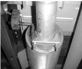
**3.** SLIP THE MUFFLER #B ONTO HEADPIPE #A NO LESS THEN 1- 1/2" AND NO MORE THEN 2". THE MUFFLER OUTLETS WILL BE LEVEL AT THE 12 O'CLOCK POSITION. THEN INSTALL HANGER #F ON THE INLET OF THE MUFFLER AND INSERT WELDED HANGER INTO RUBBER GROMMET. DO NOT TIGHTEN.
