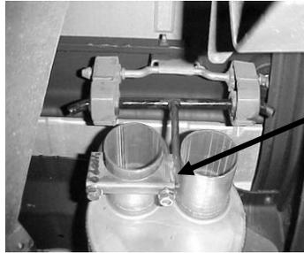
**4.** INSTALL HANGER #J ON THE DRIVER SIDE OUTLET OF MUFFLER WITH THE VERTICAL ROD IN BETWEEN THE TWO OUTLETS. DO NOT TIGHTEN
