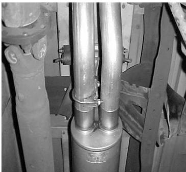
THEN, INSTALL DRIVERSIDE TAILPIPE #D. SUPPORT THE MUFFLER WITH A JACK STAND. THEN INSTALL PASSENGER SIDE OVERAXLE #C. INSERT WELDED HANGER ON TAILPIPE INTO FACTORY RUBBER GROMMET. **NOTE: SPARE TIRE MAY HAVE TO BE LOOSENED AND MOVED FOR BETTER CLEARANCES.**
