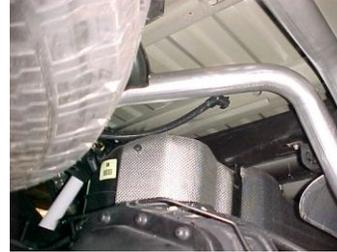
INSTALL DRIVERS SIDE TAILPIPE # D INTO MUFFLER 1 1/2" TO 2". INSERT WELDED HANGERS INTO RUBBER GROMMETS. USE CLAMP # H TO SECURE PIPE TO MUFFLER, DO NOT TIGHTEN.
