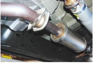
TO REMOVE YOUR STOCK EXHAUST, REMOVE IT FROM THE 2 BOLT FLANGE LOCATED JUST IN FRONT OF THE MUFFLER REMOVE HANGERS FROM RUBBER GROMMETS BY PULLING EXHAUST TOWARDS THE REAR OF THE VEHICLE, USE WD-40 TO AID IN REMOVAL, LEAVE GROMMETS IN PLACE.
