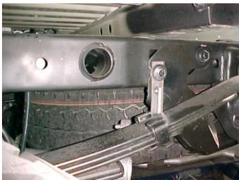
ON DRIVER SIDE: ATTACH REAR TAILPIPE HANGER #I TO FRAME BY REMOVING THE 18MM HITCH BOLT. THEN RE INSTALL BOLT WITH HANGER (IF YOU DO NOT HAVE A FACTORY HITCH USE BOLT KIT #K TO ATTACH HANGER #I & #J TO THE FRAME RAIL.
