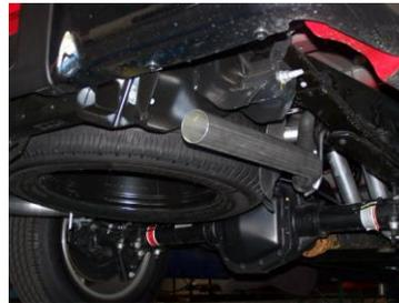
INSTALL PASSENGER SIDE TAILPIPE # C INTO MUFFLER 1 1/2" TO 2". INSERT WELDED HANGER INTO RUBBER GROMMET, USE CLAMP # H TO SECURE PIPE TO MUFFLER. DO NOT TIGHTEN. ROTATE PIPE TOWARDS DRIVERSIDE.
