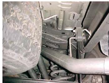
Install passenger side tailpipe # D into muffler 1-1/2" to 2", use clamp # I to secure. Do not tighten. Slide welded hanger into rubber grommet.
