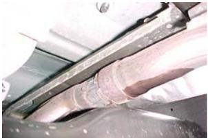
Lay out the exhaust on the floor so it looks like the drawing and compare parts with manual. To remove the stock exhaust, unclamp it just in front of the muffler. You may need to heat it up for easier removal. Leave all rubber grommets in place. Use WD-40 to aid in removal of exhaust and the hangers. Now cut off your stock tailpipe just behind the muffler.
