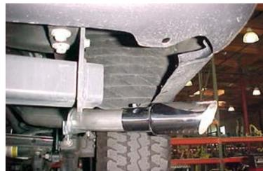
Install exit pipes # E onto tailpipes, and rotate until level.
