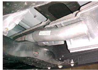
Install head pipe #A onto your existing stock front pipe and secure with clamp # G. Use a jack stand to support the converter. Do not tighten.
