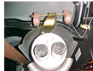
Install muffler #B onto head pipe  $1\frac{1}{2}$ " to 2" with the louvers facing towards the converter. Use a jack stand to support the muffler. Use clamp # H to secure the muffler to the head pipe. Do not tighten. Outlets should be on the bottom.
