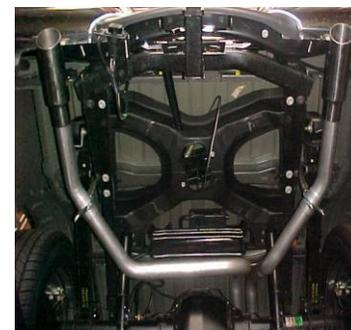
INTSTALL EXIT PIPES # F TO THE OVERAXLE TAILPIPES USE CLAMP # G TO SECURE USE ZIP TIES FOR BRAKE AND HOSE LINES TO KEEP AWAY FROM PIPES. NOW FIRMLY TIGHTEN ALL BOLTS, CLAMPS AND HANGERS. INSTALL STAINLESS TIPS.
