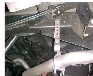
ON DRIVER SIDE MEASURE 17-1/2" FROM THE REAR OF THE FRAME FORWARD. USE HANGER # I. USE THE TOP HOLE OF THIS HANGER. USE HARDWARE PROVIDED. REPEAT FOR PASS. SIDE.
