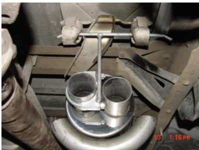
INSTALL MUFFLER #B ONTO HEADPIPE 1-1/2" TO 2". OUTLET SHOULD BE LEVEL. USE CLAMP #J TO SECURE MUFFLER TO HEADPIPE. DO NOT TIGHTEN. INSTALL REAR MUFFLER HANGER #G ONTO THE DRIVERSIDE MUFFLER OUTLET. INSERT HANGERS INTO RUBBER GROMMETS. DO NOT TIGHTEN.
