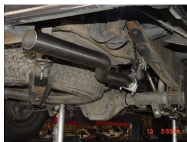
INSTALL PASSENGERSIDE TAILPIPE #C INTO MUFFLER 1-1/2" TO 2". USE CLAMP #I TO SECURE PIPE TO MUFFLER. DO NOT TIGHTEN. INSTALL STAINLESS TIPS. GO BACK AND TIGHTEN ALL CLAMPS, NUTS, AND BOLTS. USE ZIP TIES TO SECURE BRAKE, AND FUEL LINES.
