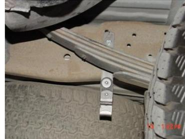
INSTALL HANGER #H ONTO FRAME OF TRUCK BY MEASURING 4" IN FRONT OF THE STOCK REAR HANGER, AND THEN 4" UP, YOU WILL USE THIS HOLE. USE THE SAME HOLE ON THE DRIVERS SIDE.
