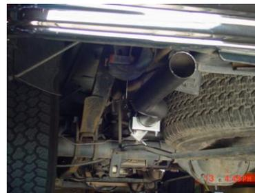
INSTALL EXIT PIPES #F ONTO TAILPIPES, ROTATE THE PIPE UNTIL IT IS AT THE PROPER LOOK FOR YOU. USE CLAMPS #I TO SECURE PIPES TOGETHER. DO NOT TIGHTEN.
