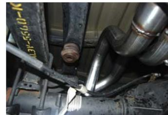
INSTALL MUFFLER # B ONTO HEADPIPE 1 1/2" TO 2". USE CLAMP # F TO SECURE MUFFLER TO HEADPIPE. DO NOT TIGHTEN. USE A JACK STAND TO HOLD UP THE MUFFLER. OUTLETS SHOULD BE LEVEL.
