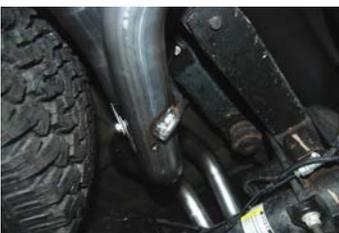
INSTALL PASS. SIDE TAILPIPE # C INTO MUFFLER 1 1/2" TO 2". INSERT HANGER INTO RUBBER GROMMET, USE CLAMP # G TO SECURE PIPE TO MUFFLER. DO NOT TIGHTEN.
