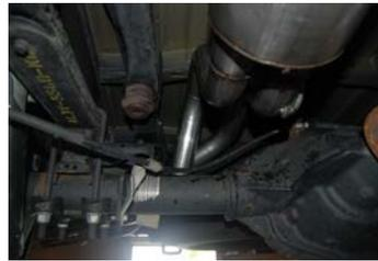
INSTALL DRIVERS SIDE TAILPIPE # D INTO MUFFLER 1 1/2" TO 2". INSERT HANGERS INTO RUBBER GROMMETS, USE CLAMP # G TO SECURE PIPE TO MUFFLER. DO NOT TIGHTEN. THE TAB ON THIS PIPE SHOULD GO ON BOTTOM OF PASSENGER SIDE PIPE USE BOLT KIT # H TO SECURE TOGETHER.
