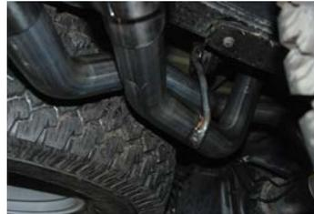
INSTALL HEADPIPE # A INTO STOCK PIPE. THE END OF THE PIPE SHOULD BE AT THE 12 O'CLOCK POSITION, ATTACH WITH FACTORY CLAMP. DO NOT TIGHTEN. INSERT WELDED HANGER INTO RUBBER GROMMET.
