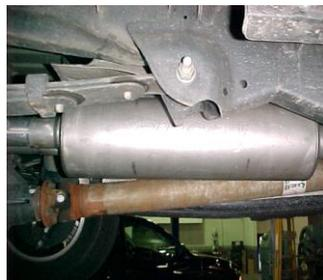
INSTALL MUFFLER # B ONTO HEADPIPE 1 1/2" TO 2". USE CLAMP # F TO SECURE MUFFLER TO HEADPIPE. DO NOT TIGHTEN. USE A JACK STAND TO HOLD UP THE MUFFLER. OUTLETS SHOULD BE LEVEL.
