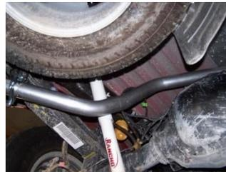
**6.** Install the driverside overaxle tailpipe #D into the muffler 1 1/2"-2". Use clamp #H to secure. DO NOT TIGHTEN. Rotate until it meets with the rubber grommet, use clamp #H to hold pipe. DO NOT TIGHTEN.
