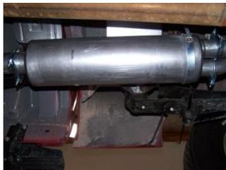
**3.** Install muffler #B onto head pipe #A 1 1/2"-2" with the louvers facing towards the converter. Use a jack stand to support the muffler. Use clamp #G to secure the muffler to the headpipe. Do not tighten. Muffler inlet is looking into the louvers.
