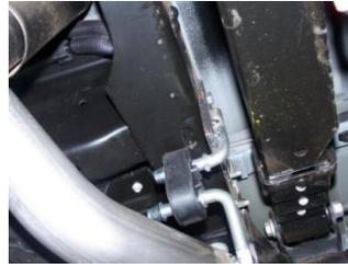
**5.** Install hanger #I into hole located approximately 19" from the rear of the frame. Use bolt kit #J to secure. DO NOT TIGHTEN. Install rubber grommet
