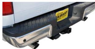
**8.** Install stainless steel tips. Clamp down. When you have everything in place, firmly tighten all bolts and clamps down securely. Use stainless steel cleaner and a Scotch Brite pad weekly to prevent tip from discoloration. Inspect all fasteners after 25-50 miles of operation and re-tighten as necessary
