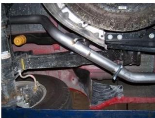
**4.** Install the passenger side overaxle tailpipe #C into the muffler 1 1/2"-2". Use clamp #H to secure tailpipe to muffler. DO NOT TIGHTEN. Insert hanger into rubber grommets.
