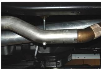
**2.** Install head pipe #A onto your existing stock front pipe and attach with clamp #G. Use a jack stand to support the converter. Insert welded hanger into rubber grommet.
