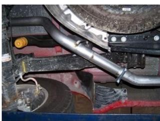
**4.** Install the passenger side overaxle tailpipe #C into the muffler 1 1/2"-2". Use clamp #H to secure tailpipe to muffler. **DO NOT TIGHTEN.** Insert hanger into rubber grommet.
