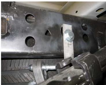
ON DRIVER SIDE: ATTACH REAR TAILPIPE HANFGER #I TO FRAME USING BOLT KIT PROVIDED
