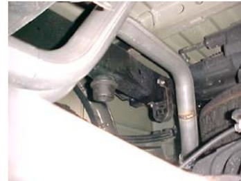
INSTALL PASSENGER SIDE TAILPIPE # C INTO MUFFLER 1 1/2" TO 2". INSERT WELDED HANGER INTO RUBBER GROMMET, USE CLAMP # H TO SECURE PIPE TO MUFFLER. DO NOT TIGHTEN. ROTATE PIPE TOWARDS DRIVERSIDE.
