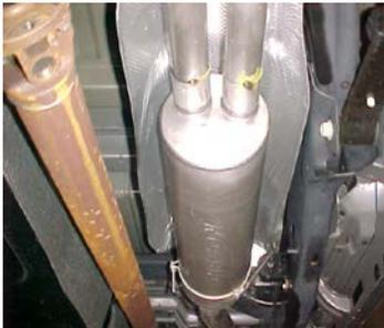
INSTALL MUFFLER # B ONTO HEADPIPE 1 1/2" TO 2". USE CLAMP # G TO SECURE MUFFLER TO HEADPIPE. DO NOT TIGHTEN. USE A JACK STAND TO HOLD UP THE MUFFLER. OUTLETS SHOULD BE LEVEL.
