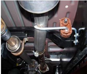
INSTALL HEADPIPE #A INTO STOCK FLANGE., ATTACH WITH BOLT KIT PROVIDED. DO NOT TIGHTEN. INSERT WELDED HANGER INTO RUBBER GROMMET.
