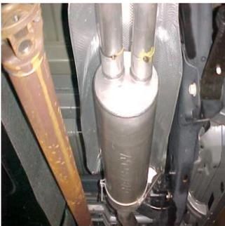
INSTALL MUFFLER # B ONTO HEADPIPE 1 1/2" TO 2". USE CLAMP # G TO SECURE MUFFLER TO HEADPIPE. DO NOT TIGHTEN. USE A JACK STAND TO HOLD UP THE MUFFLER. OUTLETS SHOULD BE LEVEL.
