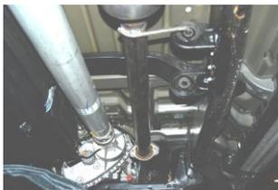
INSTALL HEADPIPE #A INTO STOCK PIPE. THE END OF THE PIPE SHOULD BE AT THE 12 O'CLOCK POSITION, ATTACH WITH BOLT KIT # L. DO NOT TIGHTEN. INSERT WELDED HANGER INTO RUBBER GROMMET. REMOVE THE HANGER FROM THE FRAME & RELOCATE TO THE HOLES JUST TO THE LEFT OF THE OTHER HOLES YOU WILL NEED TO PRY THE INSERTS OUT & RE-INSTALL SEE PHOTO
