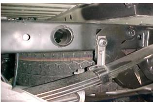
ON DRIVER SIDE: ATTACH REAR TAILPIPE HANGER #I TO FRAME BY REMOVING THE 18MM HITCH BOLT. THEN RE INSTALL BOLT WITH HANGER. (IF YOU DO NOT HAVE A FACTORY HITCH USE BOLT KIT #K TO ATTACH HANGER #I TO THE FRAME RAIL.
