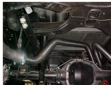
FINALLY AFTER TIGHTENING ALL CLAMPS FROM FRONT TO BACK AND MAKING SURE OF CLEARANCES,
