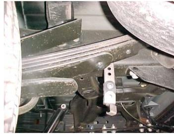
NEXT INSTALL DRIVERS SIDE OVERAXLE PIPE #D INTO MUFFLER 1 1/2" TO 2". USE CLAMP #I TO SECURE PIPE TO MUFFLER. DO NOT TIGHTEN. ROTATE PIPE UNTIL IT TOUCHES HANGER. USE CLAMP #I TO HOLD PIPE TO HANGER DO NOT TIGHTEN.
