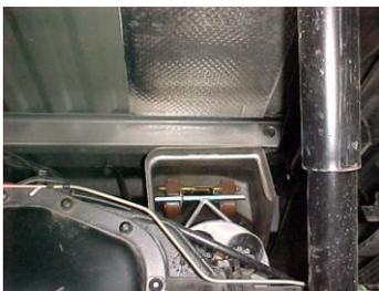
NEXT, LOCATE THE SLOTTED HOLES LOCATED APPROXIMATELY 16" FROM THE REAR OF THE FRAME. MOUNT THE 10" STRAP HANGERS #J INTO THESE SLOTS USING THE HARDWARE KIT # J. MOUNT USING THE 2<sup>ND</sup> HOLE FROM THE TOP.
