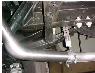
INSTALL MUFFLER #B ONTO HEADPIPE 1 1/2" TO 2". MUFFLER OUTLETS SHOULD BE ON TOP. ROTATE UNTIL LEVEL. SUPPORT MUFFLER WITH A JACK STAND. NEXT, INSTALL FRONT MUFFLER HANGER #F INTO RUBBER GROMMETS, LOCATED NEXT TO MUFFLER INLET. THIS CLAMP WILL ALSO BE USED TO SECURE MUFFLER TO HEADPIPE. DO NOT TIGHTEN.
