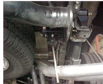
NEXT, INSTALL DRIVERS SIDE TAILPIPE # D INTO MUFFLER 1 1/2"-2". INSERT WELDED HANGER INTO RUBBER GROMMET, BOLT TAILPIPES TOGETHER WITH BOLT KIT # K. DRIVERS SIDE TAB WILL BE ON THE BOTTOM.
