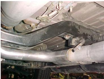
INSTALL Y-PIPE # A & M ONTO STOCK FLANGES USE YOUR STOCK HARDWARE TO SECURE INSERT WELDED HANGER INTO RUBBER GROMMET, DO NOT TIGHTEN.
