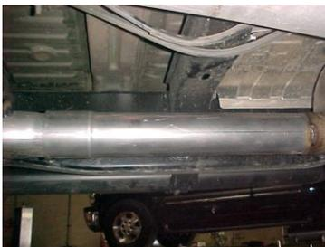
INSTALL EXTENSION PIPE #L ONTO HEADPIPE. INSERT WELDED HANGER INTO GROMMET. USE CLAMP # G TO SECURE. DO NOT TIGHTEN.
