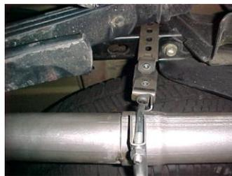
ON THE DRIVERS SIDE MEASURE APPROX. 17" FROM THE REAR OF THE FRAME USE THIS 1" HOLE TO BOLT HANGER # K USING THE TOP HOLE ON HANGER & HARDWARE PROVIDED, REPEAT FOR PASSENGER SIDE.
