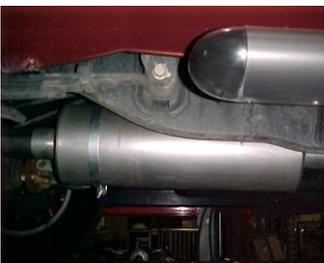
NEXT, INSTALL RESONATOR # B 1 1/2"-2" ONTO Y-PIPE USE CLAMP # I TO SECURE PIPES TOGETHER, DO NOT TIGHTEN.
