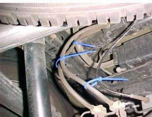
WE HAVE PROVIDED ZIP TIES, SO YOU CAN ZIP TIE BRAKE LINES, FUEL LINES, ETC AWAY FROM EXHAUST PIPES.
