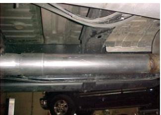
INSTALL MUFFLER # C ONTO YOUR RESONATOR 1 1/2" -2". USE CLAMP # I TO SECURE MUFFLER TO THE PIPE, DO NOT TIGHTEN.
