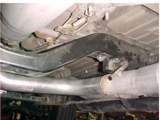
INSTALL Y-PIPE # A & O ONTO STOCK FLANGES USE YOUR STOCK HARDWARE TO SECURE INSERT WELDED HANGER INTO RUBBER GROMMET, DO NOT TIGHTEN. USE CLAMP #J TO SECURE PIPES TOGETHER. DO NOT TIGHTEN.
