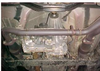
NEXT, UN-BOLT YOUR EXHAUST FROM THE 2-BOLT FLANGES LOCATED JUST BEHIND YOUR FACTORY CATALYTIC CONVERTERS, DO NOT DISCARD YOUR FACTORY GASKETS AND HARDWARE YOU WILL RE-USE IT.
