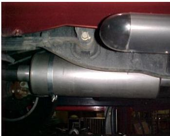
INSTALL MUFFLER # C ONTO YOUR RESONATOR 1 1/2" -2". USE CLAMP # I TO SECURE MUFFLER TO THE PIPE, DO NOT TIGHTEN.
