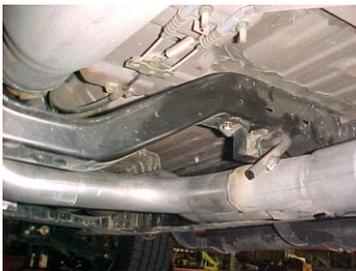
INSTALL Y-PIPE # A & O ONTO STOCK FLANGES USE YOUR STOCK HARDWARE TO SECURE INSERT WELDED HANGER INTO RUBBER GROMMET, DO NOT TIGHTEN. USE CLAMP # J TO SECURE PIPES TOGETHER. DO NOT TIGHTEN.
