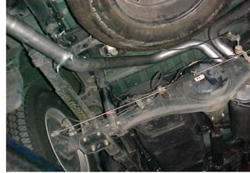
INSTALL THE DRIVERSIDE OVER AXLE TAILPIPE #C ONTO MUFFLER 1-1/2" TO 2" USE CLAMP # I TO SECURE PIPE TO MUFFLER, DO NOT TIGHTEN.
