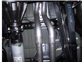
6. Install the passenger side over axle tailpipe #F to the extension pipe 1.5"-2". Using clamp #I to secure pipes together. Do not tighten. Insert welded hanger into rubber grommet.
