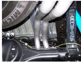
7. Install driver side over axle tailpipe #G onto extension pipe. Use clamp #I to secure the pipe. Do not tighten.
