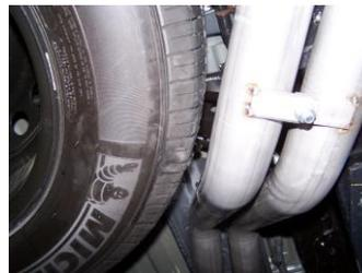
8. Use bolt kit #J to secure tabs. Make sure driver side tab is on the bottom. (You may need to loosen up the spare tire and move it over for better clearance.)
