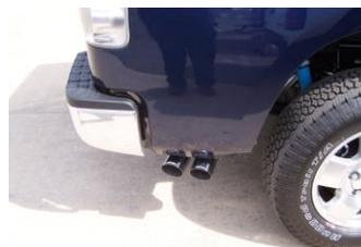
9. Install stainless steel tips. Clamp down. When you have everything in place, firmly tighten all bolts and clamps down securely. Use stainless steel cleaner and a Scotch Brite pad weekly to prevent tip from discoloration. Inspect all fasteners after 25-50 miles of operation and re-tighten as necessary.
