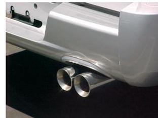
**"MAKE SURE HAVE A MINIMUM OF A 1" ON ALL PIPES FROM ALL RUBBER BRAKE LINES, TIRES, SHOCKS, FUEL LINES, ETC.**
