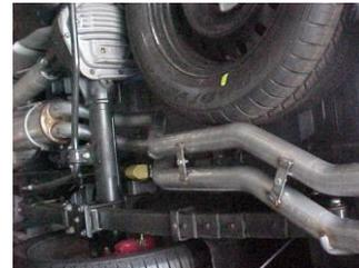
Install the driver side over axle tailpipe #D into the muffer 1-1/2" to 2". Use clamp #H to secure tailpipe to muffer. Use bolt kit #I to secure tailpipes #D & E together. Driver side tailpipe will have tab on bottom. Do not tighten.
