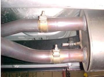
Lay out the exhaust on the floor so it looks like the drawing and compare parts with manual. To remove the stock exhaust un-clamp it just in front of the muffer. Leave all rubber grommets in place. Use WD-40 to aid in removal of exhaust and the hangers.
