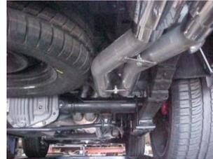
Install the passenger side over axle tailpipe #E into the muffer 1-1/2" to 2" and attach using clamp #H. Insert hanger into rubber grommet. Do not tighten.
