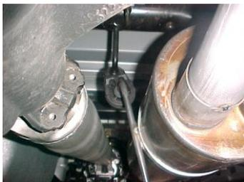
Slide band clamp #G onto muffer #C. Insert hangers into rubber grommets. Do not tighten.
