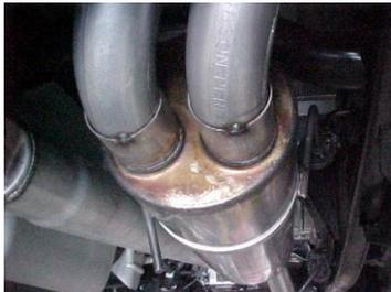
Install muffer #C onto head pipes 1-1/2" to 2" with the louvers facing towards the converter. The inlets and outlets of the muffer will be on the bottom. Use a jack stand to support the muffer. Use clamp #H to secure the muffer to the head pipes. Do not tighten. Muffer inlet is looking into the louvers.
