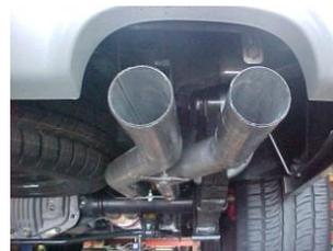
Install the stainless tips. Clamp down. To clean your stainless tips use any stainless cleaner or a Scotch Brite pad. Now go back and tighten all clamps, nuts and bolts. Start from the front and work back.
