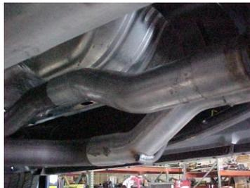
Install head pipe #A onto passenger side stock pipe and insert hanger into rubber grommet. Next install driver side head pipe #B onto drivers side factory pipe. Use clamp #H to secure pipes to factory pipes. Do not tighten.
