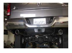
7. Install exit pipes #E onto tailpipes use clamp # F to secure together. After everything is installed begin to tighten all connections starting from the furthest forward connection. Items will move as you tighten. Be sure to check all clearance.
