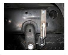
5. Next install drivers side rear hanger and grommet with bolt kit on the outside of the driver side frame rail. Use the factory drilled hole just forward of the large hole seen in the photo above.
