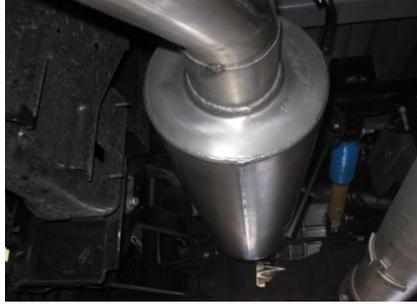
3. Install muffler #B onto headpipe 1.5" to 2" muffler outlets should be on top and level use clamp #G to secure together. Do not tighten. Insert hangers into rubber grommets
