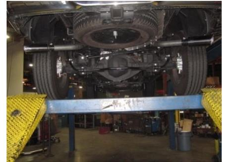
7. Install exit pipes #E onto tailpipes use clamp # F to secure together. After everything is installed begin to tighten all connections starting from the furthest forward connection. Items will move as you tighten. Be sure to check all clearance.
