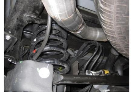
4. Next install Drivers side overaxle tailpipe #C into muffler 1.5" to 2" use clamp #F to secure pipe to muffler do not tighten
