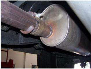
**1.** To remove the stock exhaust remove it from the clamp located in front of your stock muffler. Use WD-40 to aid in removal of hangers from rubber grommets. Next measure 30" from end of pipe towards front of the vehicle and cut here.
