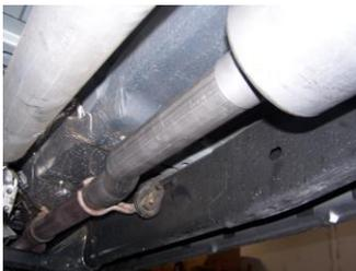
**2.** Insert muffer assembly #A into headpipe head pipe and attach with clamp #B. **DO NOT TIGHTEN** Use a jack stand to support the muffer assembly.
