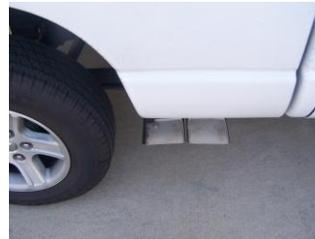
**4.** Install stainless steel tips. Clamp down. When you have everything in place, firmly tighten all bolts and clamps down securely. Use stainless steel cleaner and a Scotch Brite pad weekly to prevent tip from discoloration. Inspect all fasteners after 25-50 miles of operation and re-tighten as necessary
