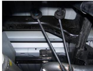
**3.** Insert welded hangers into rubber grommets.
