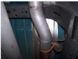
3. Install headpipe #A onto your existing stock headpipe and secure with clamp #G. Use a jack stand to support the converter.
