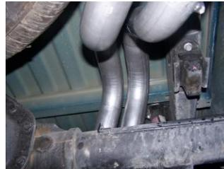
7. Install the driver side over axle tailpipe #C into the muffler 1.5-2" Use clamp #F to secure tailpipe to muffler. Do not tighten.
