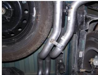
8. Attach tailpipes together with bolt kit #I. Do not tighten. Driver side tabs will be on the bottom.
