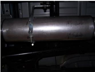
4. Install muffler #B onto headpipe #A 1.5-2" with the louvers facing towards the converter. Use a jack stand to support the muffler. Use clamp #E to secure the muffler to the headpipe. Do not tighten. Muffler inlet is looking into the louvers.
