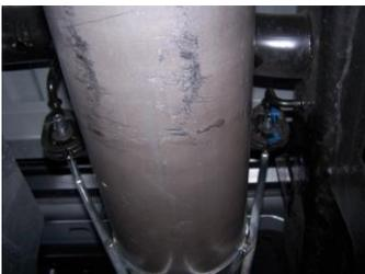
5. Slide band clamp #H onto muffler #B and attach with bolt kit #J. Do not tighten. Insert hangers into rubber grommets.
