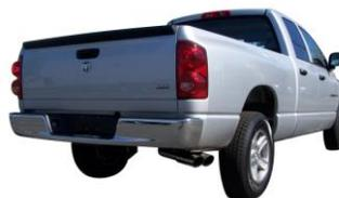
9. Install stainless steel tips. Clamp down. When you have everything in place, firmly tighten all bolts and clamps down securely. Use stainless steel cleaner and a Scotch Brite pad weekly to prevent tip from discoloration. Inspect all fasteners after 25-50 miles of operation and re-tighten as necessary.
