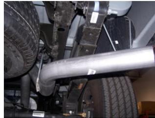
6. Install the passenger side over axle tailpipe #D into the muffler 1.5-2". Use clamp #F to secure tailpipe to muffler. Do not tighten.
