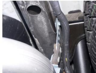
**5.** Use the hole 19½" from the rear of the frame to attach the 10" hanger #G with bolt kit #L. Use the second hole from the top.
