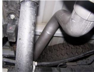
**4.** Install passenger side tailpipe #C into muffler 1½-2". Use clamp #G to secure tailpipe to muffler. DO NOT TIGHTEN. Insert welded hanger into rubber grommet.
