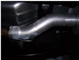
**2.** Install head pipe #A onto your existing stock front pipe and attach with clamp #I. Use a jack stand to support the converter. Insert welded hanger into rubber grommet.
