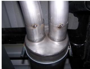
**6.** Install driver side tailpipe #D 1½-2" into muffler and use clamp #G to secure to muffler. Attach clamp #G to hold up to the hanger #H. DO NOT TIGHTEN.
