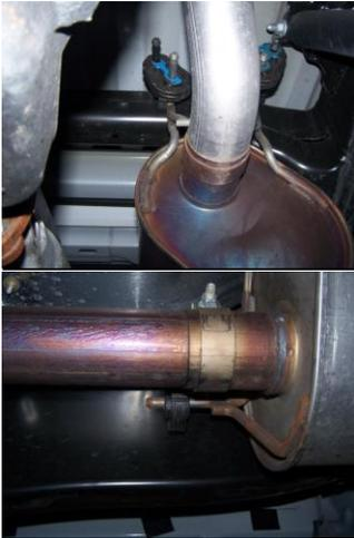
**1.** To remove the stock exhaust remove it from located in front of the new muffler. Disengage the welded hangers using WD-40 from the OEM rubber grommets. Do not damage or remove the rubber grommets as you will re-use them to mount your new system. Now, cut off tailpipe and remove exhaust.
