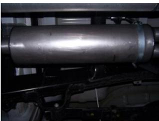
**3.** Install muffler #B onto head pipe #A 1½"-2" with the louvers facing towards the converter. Use a jack stand to support the muffler. Use clamp #I to secure the muffler to the headpipe. Slide band clamp onto muffler and insert welded hangers into rubber grommets. Attach with bolt kit #K. DO NOT TIGHTEN. Muffler inlet is looking into the louvers.
