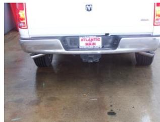
GIBSON EXHAUST systems are designed on a factory stock vehicle. Any aftermarket products installed could increase the sound levels of this Exhaust. **Make sure there is a 1" clearance from ALL rubber brake lines, shock boots, fuel lines, tires, etc to prevent heat related damage or fire.**
