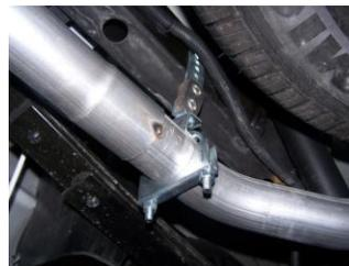
**7.** Install exit pipes #E, use clamps #G to secure to tailpipes. DO NOT TIGHTEN.
