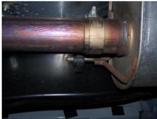
**2.** Install head pipe #A onto your existing stock front pipe and attach with clamp #H. Use a jack stand to support the converter. Insert welded hanger into rubber grommet.
