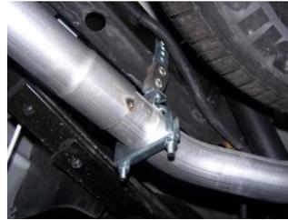
**7.** Install exit pipes #E, use clamps #G to secure to tailpipes. **DO NOT TIGHTEN.** Roll pipes until you have the angle you desire.
