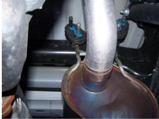
**1.** To remove the stock exhaust remove it from in front of the stock muffler. Disengage the welded hangers using WD-40 from the OEM rubber grommets. Do not damage or remove the rubber grommets as you will re-use them to mount your new system. Now, cut off tailpipe and remove exhaust.
