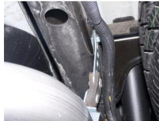
**5.** Use the hole 19½" from the rear of the frame to attach the 10" hanger #F with bolt kit #M. Use the third hole from the top on the hanger.
