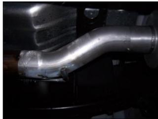
**3.** Install muffler #B onto head pipe #A 1½"-2" with the louvers facing towards the converter. Use a jack stand to support the muffler. Use clamp #H to secure the muffler to the headpipe. Slide band clamp #I onto muffler and insert welded hangers into rubber grommets. Attach with bolt kit #K. **DO NOT TIGHTEN.** Muffler inlet is looking into the louvers.
