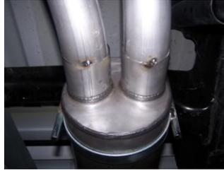
**6.** Install driver side tailpipe #D 1½-2" into muffler and use clamp #G to secure to muffler. Attach clamp #G to hold up to the hanger #F. **DO NOT TIGHTEN.**
