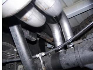
**4.** Install driver side tailpipe #C into muffler. Use clamp # F to secure. DO NOT TIGHTEN.
