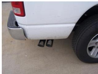
**6.** Install stainless steel tips. Clamp down. When you have everything in place, firmly tighten all bolts and clamps down securely. Use stainless steel cleaner and a Scotch Brite pad weekly to prevent tip from discoloration. Inspect all fasteners after 25-50 miles of operation and re-tighten as necessary
