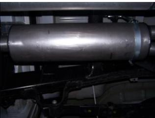
**3.** Install muffler #B onto head pipe #A 1½"-2" with the louvers facing towards the converter. Use a jack stand to support the muffler. Use clamp #G to secure the muffler to the headpipe. Slide band clamp onto muffler and insert welded hangers into rubber grommets. Attach with bolt kit #J. DO NOT TIGHTEN. Muffler inlet is looking into the louvers.
