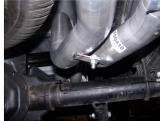
**5.** Install passenger side tailpipe #D into muffler, attach with clamp #F. Insert welded hanger into rubber grommet. DO NOT TIGHTEN. Use bolt kit #I to attach the two tailpipes together. The driver side tab will be on the bottom.
