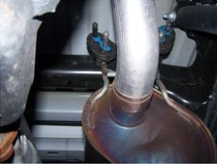
**1.** To remove the stock exhaust un-clamp the tailpipe just after the stock muffler. Then un-clamp the stock muffler. Leave all rubber grommets in place. Use WD-40 to aid in removal of exhaust.
