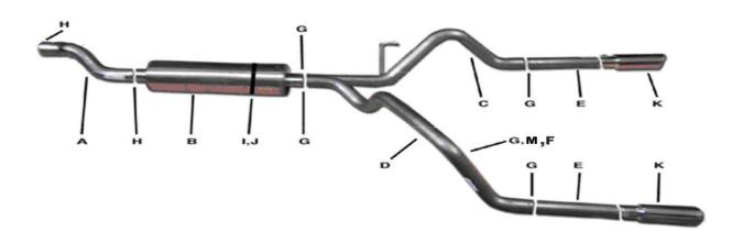
TO REMOVE STOCK EXHAUST, UNCLAMP JUST IN FRONT OF MUFFLER
