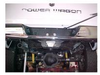
MEASURE 19 1/2" FROM THE REAR OF THE FRAME AND USE THIS HOLE AND BOLT ON HANGER #F. USE THE 1<sup>ST</sup>. HOLE FROM THE TOP. IT WILL BOLT ON THE INSIDE OF THE FRAME.
