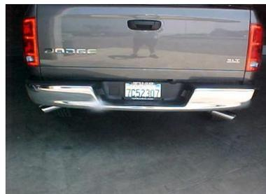
INSTALL THE STAINLESS TIPS. TO CLEAN TIPS USE ANY STAINLESS CLEANER AND A SCOTCH BRITE PAD. NOW GO BACK AND TIGHTEN ALL CLAMPS, NUTS AND BOLTS STARTING FROM THE FRONT AND WORKING BACK.
