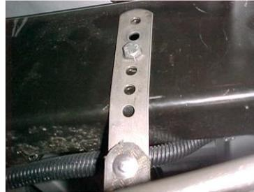
MEASURE 19 1/2" FROM THE REAR OF THE FRAME AND USE THIS HOLE AND BOLT ON HANGER #H. USE THE 2<sup>ND</sup> HOLE FROM THE TOP.
