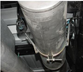
INSTALL MUFFLER #B ONTO HEADPIPE 1-1/2" TO 2". USE CLAMP #I TO SECURE THE MUFFLER TO THE HEADPIPE. DO NOT TIGHTEN. SLIDE BAND CLAMP #J ONTO THE MUFFLER AND INSERT THE WELDED HANGER INTO THE RUBBER GROMMET. ATTACH WITH BOLT KIT #K.
