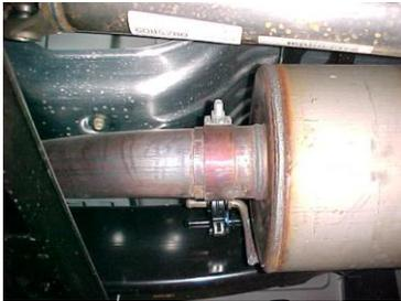
**TO REMOVE STOCK EXHAUST REMOVE IT FROM THE CLAMP LOCATED IN FRONT OF YOUR STOCK MUFFLER. NOW CUT OFF YOUR STOCK TAILPIPE JUST BEHIND THE MUFFLER AND REMOVE. LEAVE ALL RUBBER GROMMETS ON THE HANGER. USE WD-40 TO AID IN REMOVAL OF EXHAUST AND HANGERS.**
