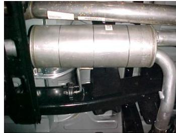
INSTALL MUFFLER ASSEMBLY #A ONTO STOCK PIPE 1-1/2" TO 2". SLIDE WELDED HANGERS INTO RUBBER GROMMETS YOU MAY NEED TO ADJUST WELDED HANGERS TO FIT INTO YOUR GROMMETS. USE A JACKSTAND TO SUPPORT YOUR MUFFLER. USE CLAMP #B TO SECURE IT TO YOUR HEADPIPE. DO NOT TIGHTEN
