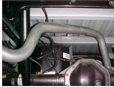
SPARE TIRE MAY NEED TO BE LOOSENED AND PUSHED TO THE REAR OF THE TRUCK FOR BETTER CLEARANCE.
