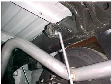
INSTALL PASSENGER SIDE TAILPIPE #C INTO MUFFLER 1-1/2" TO 2". USE CLAMP #G TO SECURE TAILPIPE TO MUFFLER. INSERT WELDED HANGER INTO RUBBER GROMMET. DO NOT TIGHTEN.
