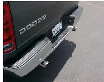
NOW GO BACK AND TIGHTEN ALL CLAMPS, NUTS AND BOLTS STARTING FROM THE FRONT AND WORKING BACK. INSTALL STAINLESS TIPS. USE ZIP TIES FOR BRAKE LINES, WIRES, ETC.
