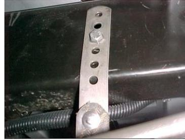
MEASURE 19 1/2" FROM THE REAR OF THE FRAME AND USE THIS HOLE AND BOLT ON HANGER #F. USE THE 3<sup>RD</sup> HOLE FROM THE TOP.
