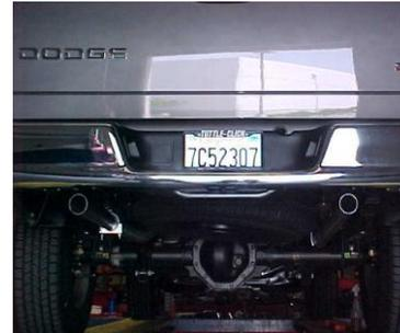
INSTALL THE EXIT PIPES #E ONTO THE TAILPIPES USING CLAMPS #G. ROLL THE PIPES UNTIL YOU HAVE THEM AT THE ANGLE YOU DESIRE.
