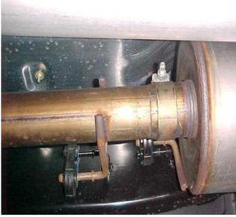
YOU MAY NEED TO HEAT IT UP FOR EASIER REMOVAL. LEAVE ALL RUBBER GROMMETS IN PLACE. USE WD-40 FOR REMOVAL OF HANGERS.
