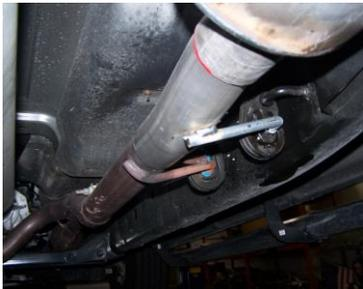
INSTALL HEADPIPE #A ONTO YOUR EXISTING STOCK FRONT PIPE AND SECURE WITH CLAMP #K. USE A JACKSTAND TO SUPPORT THE CONVERTER. INSERT WELDED HANGER INTO RUBBER GROMMET. DO NOT TIGHTEN.
