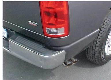
INSTALL THE STAINLESS TIPS. NOW GO BACK AND TIGHTEN ALL CLAMPS, NUTS AND BOLTS STARTING FROM THE FRONT AND WORKING BACK. TO CLEAN TIPS USE ANY STAINLESS CLEANER.
