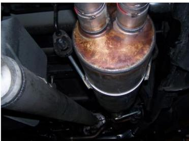
INSTALL MUFFLER #B ONTO HEADPIPE 1-1/2" TO 2". USE CLAMP #G TO SECURE THE MUFFLER TO THE HEADPIPE. DO NOT TIGHTEN. SLIDE BAND CLAMP #H ONTO THE MUFFLER AND INSERT THE WELDED HANGERS INTO THE RUBBER GROMMETS. ATTACH WITH BOLT KIT #J.
