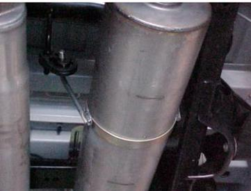
INSTALL MUFFLER #B ONTO HEADPIPE 1-1/2" TO 2". USE CLAMP #H TO SECURE THE MUFFLER TO THE HEADPIPE. DO NOT TIGHTEN. SLIDE BAND CLAMP #I ONTO THE MUFFLER AND INSERT THE WELDED HANGER INTO THE RUBBER GROMMET. ATTACH WITH BOLT KIT #L.
