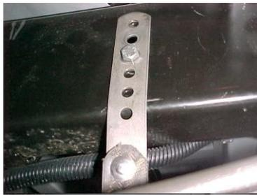
MEASURE 19 1/2" FROM THE REAR OF THE FRAME AND ON THE DRIVERS SIDE USE THIS HOLE AND BOLT ON HANGER #F. USE THE 3<sup>RD</sup> HOLE FROM THE TOP.
