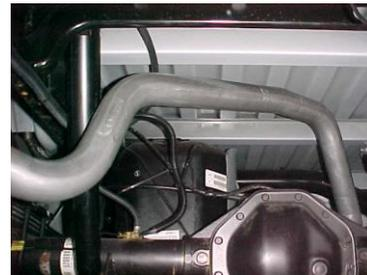
INSTALL DRIVER SIDE TAILPIPE #D INTO MUFFLER 1-1/2" TO 2" AND USE CLAMP #G TO SECURE THE MUFFLER. DO NOT TIGHTEN. USE CLAMP #G TO HOLD PIPE UP TO THE HANGER #F.
