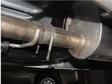
**TO REMOVE STOCK EXHAUST UNCLAMP IT FROM THE CLAMP LOCATED JUST IN FRONT OF YOUR STOCK MUFFLER. YOU MAY NEED TO HEAT IT UP WITH A TORCH TO REMOVE IT. NOW CUT OFF YOUR STOCK TAILPIPE JUST BEHIND THE MUFFLER AND REMOVE. LEAVE ALL RUBBER GROMMETS ON THE HANGER. USE WD-40 TO AID IN REMOVAL OF EXHAUST AND HANGERS.**
