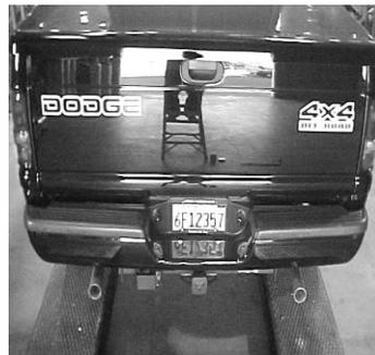
**MAKE SURE YOU HAVE A 1" CLEARANCE ON ALL PIPES FROM BRAKE LINES, FUEL LINES, SHOCKS, TIRES, ETC..**
