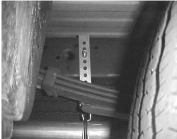
REPEAT THE SAME FOR THE DRIVERSIDE OVERAXLE TAILPIPE # D. IF YOU CAN NOT GET THE PASSENGER TAILPIPE TO CLEAR REMOVE SPARE TIRE AND ROTATE THE MUFFLER TOWARDS THE DRIVERSIDE AND ALIGN TAILPIPES AWAY FROM THE SHOCK.
