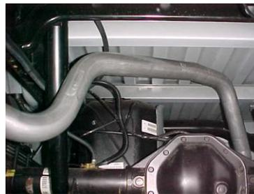
INSTALL DRIVER SIDE TAILPIPE #D INTO MUFFLER 1-1/2" TO 2" AND USE CLAMP #G TO SECURE TO THE MUFFLER. DO NOT TIGHTEN. ATTACH CLAMP #G TO HOLD PIPE UP TO THE HANGER #H. DO NOT TIGHTEN.
