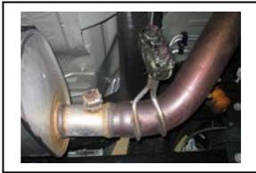
2. To remove your factory exhaust first cut off your tailpipe just behind the stock muffler. Use WD-40 to aid in removal of your factory grommets. Do not discard you will reuse them.
