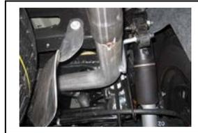
6. Install passenger side overaxle tailpipe #c into muffler 1.5" to 2" insert welded hangers into rubber grommets
