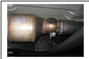
4. Install head pipe #A onto factory pipe. Use your factory clamp to secure. Insert welded hangers into rubber grommets. Do not tighten.
