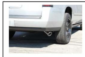
8. Install stainless steel tip. Clamp down. When you have everything in place, firmly tighten all bolts and clamps down securely. Use stainless steel or aluminum cleaner to polish tips. Inspect all fasteners after 25-50 miles of operation and re-tighten as necessary. You may need to cut your stock tail pipe back to get your tip to fit correctly.
