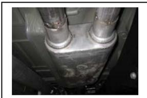
5. Install muffler #B onto head pipe #A 1 1/2"-2" with the louvers facing towards the converter. Use a jack stand to support the muffler. Use clamp #g to secure the muffler to the head pipe. Do not tighten. Muffler inlet is looking into the louvers.
