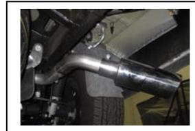
9. Install exit pipes #e onto your tailpipes adjust to your personal look use clamps #h to secure do not tighten.
