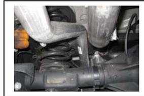
8. Install overaxle tailpipe #d into muffler 1.5" to 2" insert welded hangers into rubber grommets use clamp #h to secure do not tighten
