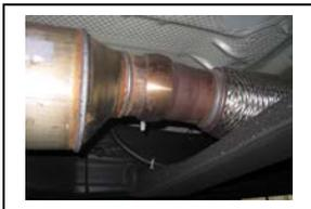
3. Next remove the rest of your stock exhaust from the clamp located in front of the muffler.
