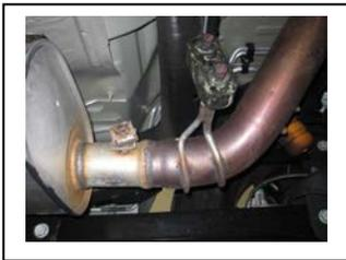
3. Remove the rest of your stock exhaust from the clamp located in front of your stock muffler you will re use it.
