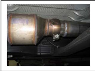
4. Install head pipe #A onto factory pipe re-use your factory clamp to secure insert welded hanger into rubber grommet. Do not tighten
