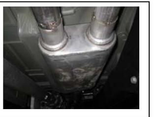
5. Install muffler #B onto head pipe #A 1 1/2"-2" with the louvers facing towards the converter. Use a jack stand to support the muffler. Use clamp #f to secure the muffler to the head pipe. Do not tighten. Muffler inlet is looking into the louvers.
