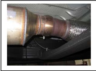
2. To remove your stock exhaust cut your tailpipe just behind the muffler use wd-40 to aid in the removal of the rubber grommets you will re use them.
