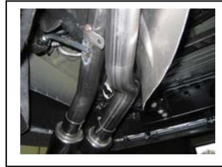
6. Next install passenger side tailpipe #c into muffler 1.5"to rubber grommet use clamp #g to secure together do not tighten.
