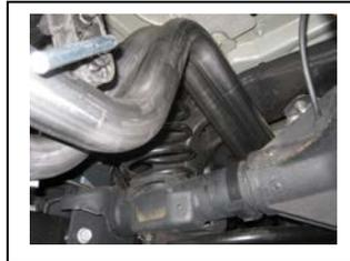
7. Next install driver side overaxle tailpipe #d into muffler. Insert welded hanger use clamp #g to secure bolt tailpipes together with bolt kit provided.
