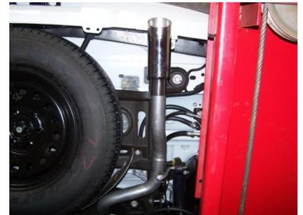
5. Next install drivers side rear hanger and grommet with bolt kit provided see picture the hanger goes on the outside of the frame and bolts through the whole frame
