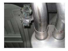
4.Next install Drivers side overaxle tailpipe #C into muffler 1.5" to 2" insert welded hanger into rubber grommet use clamp # F to secure pipe to muffler do not tighten
