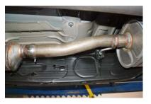
2. To remove stock exhaust, unclamp it at the connection behind the Y-pipe. Make sure to leave all rubber grommets in the factory location. You will re-use clamp. For easier removal of exhaust, cut behind the muffler. Use WD-40 to remove hangers from grommets.
