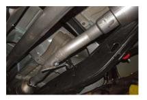
3. Install Headpipe #A onto the factory headpipe. Use the stock clamp and do not tighten. Install hanger into rubber grommet.
